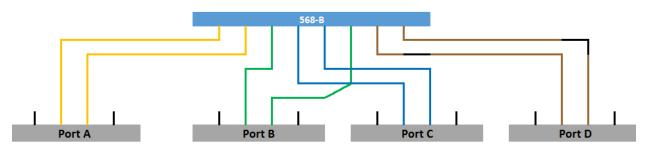
The DLC8 card has 2 RJ45s. Each Connector supports 4 phones.
